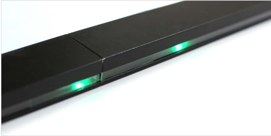
Figure 15: LEDs Showing a Secured Connection between Bars
