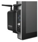
Annotating, erasing, and scrolling up & down the presentation slides will be an ease with the C2C Pen, the C2C pen holder receives the C2C Pen signals, provides a secure pen storage and charges the pen at the same time. The C2C OPS module is an Intel® OPS compliant mini PC for Interactive Touch Displays and Digital Signage applications.
