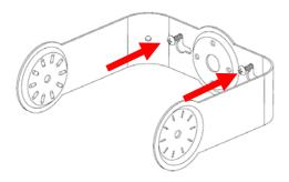
NOTE: Do not position the top of bracket closer than 140mm to cornice.
